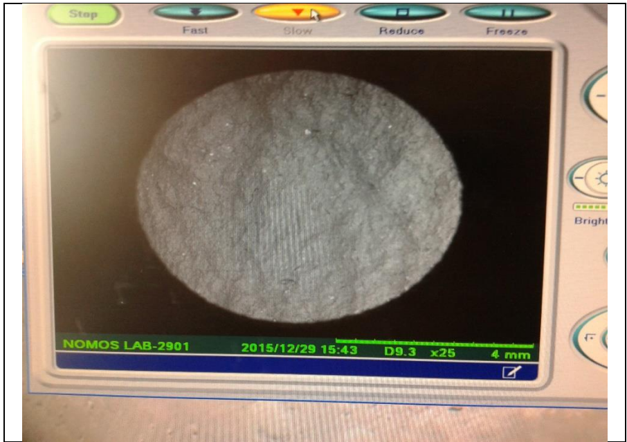
Overall view of the chip, with white specks within a grey matrix
