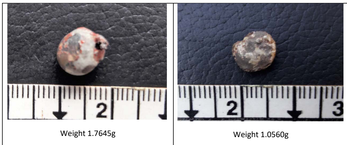
Fig. 1. Metallic buttons recovered from two-stage leach of 1kg Ema bulk sample
