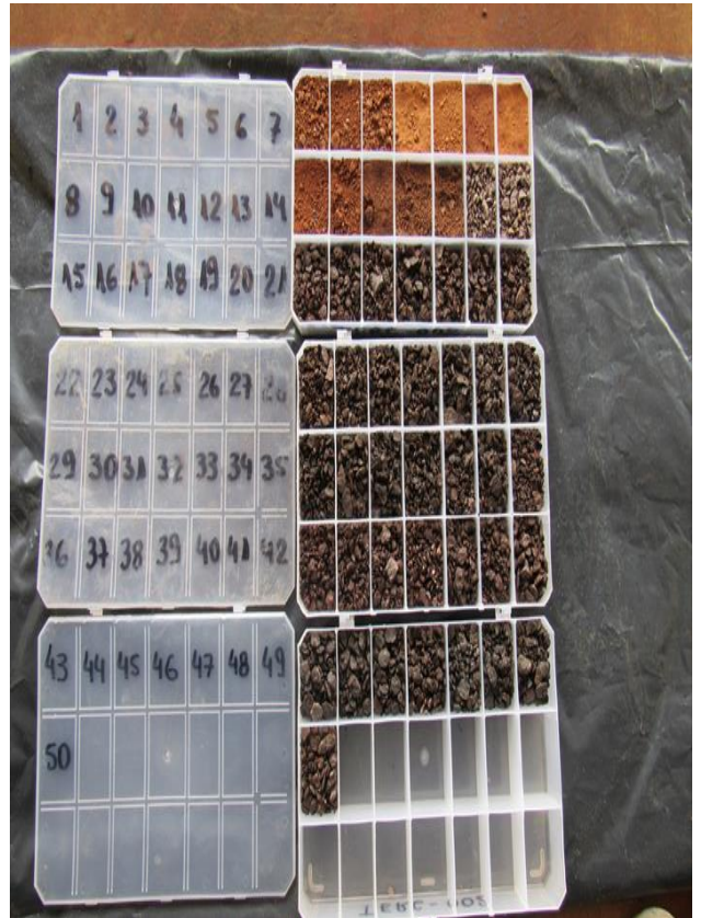
Fig. 4 One metre RC chip samples from hole TERC 02, showing fresh gabbro from 13m.
