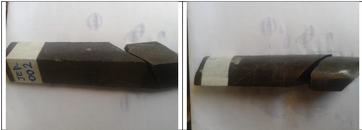
¼ core of JED_006 from where a thin (2mm) chip was collected and inspected by the SEM at Nomos.
