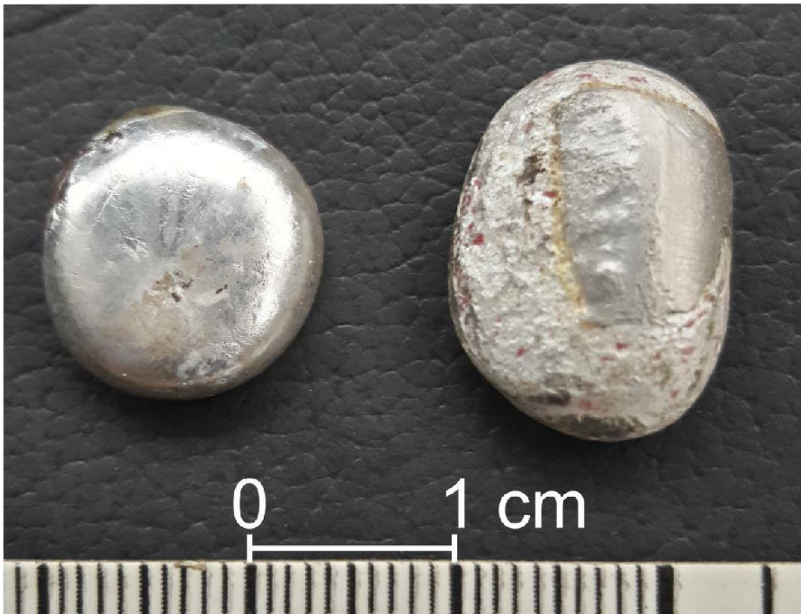
Figure 2. Buttons recovered by pyrometallurgical extraction process weighing 6.9467g and 10.4836g
