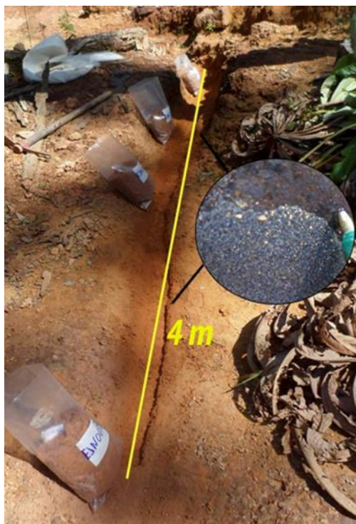
Photo 2. Raimundão, – gold in the stockwork in volcanic tuffs with intercalation of ferruginous sandstone.
