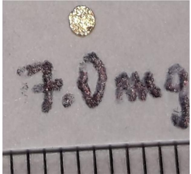
Fig. 4. Gold button recovered from 500g sample (75 of the slag utilised) (scale divisions are 1mm)
