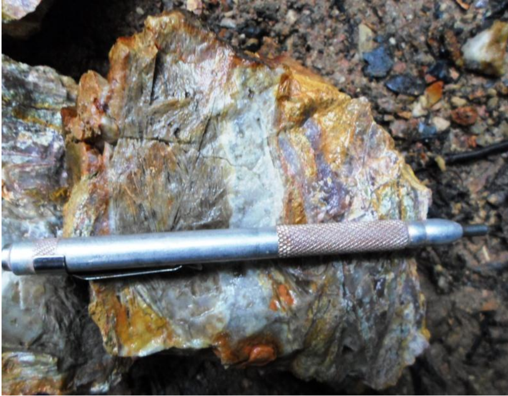
Photo 6- Sample GUN019 -from the Guida creek bed - pseudo acicular quartz
