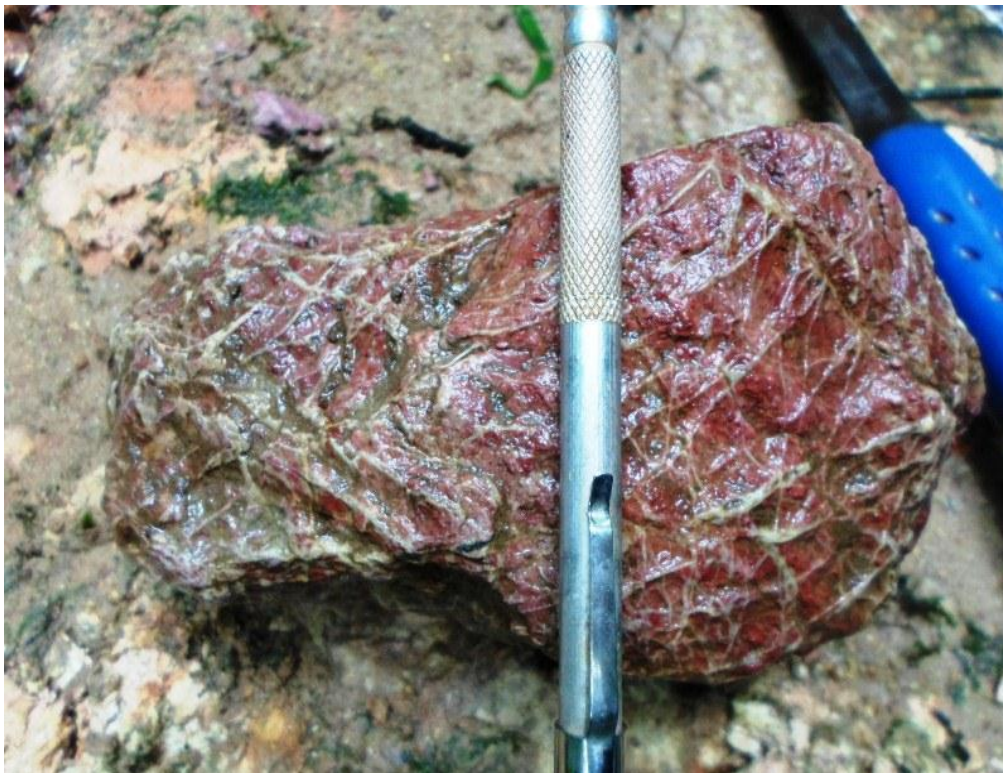
Photo 11 - Sample from the Guida creek bed – brecciated fine-grained silica mass
