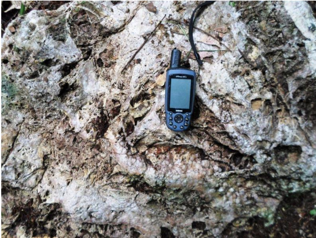
Photo 2- Exposure-location 217694E/9260309N elev. 160 m – lattice-bladed calcite replaced by quartz
