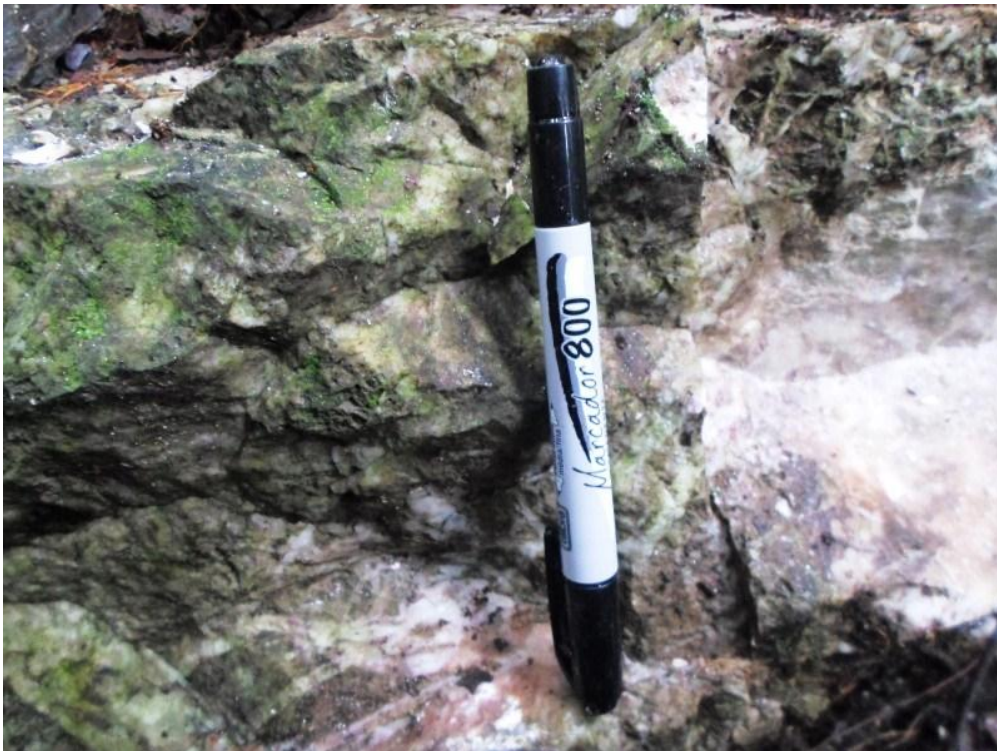
Photo 3- GUR005- location 217694E/9260309N elev. 160 m – lattice-bladed calcite replaced by quartz, epidote and adularia
