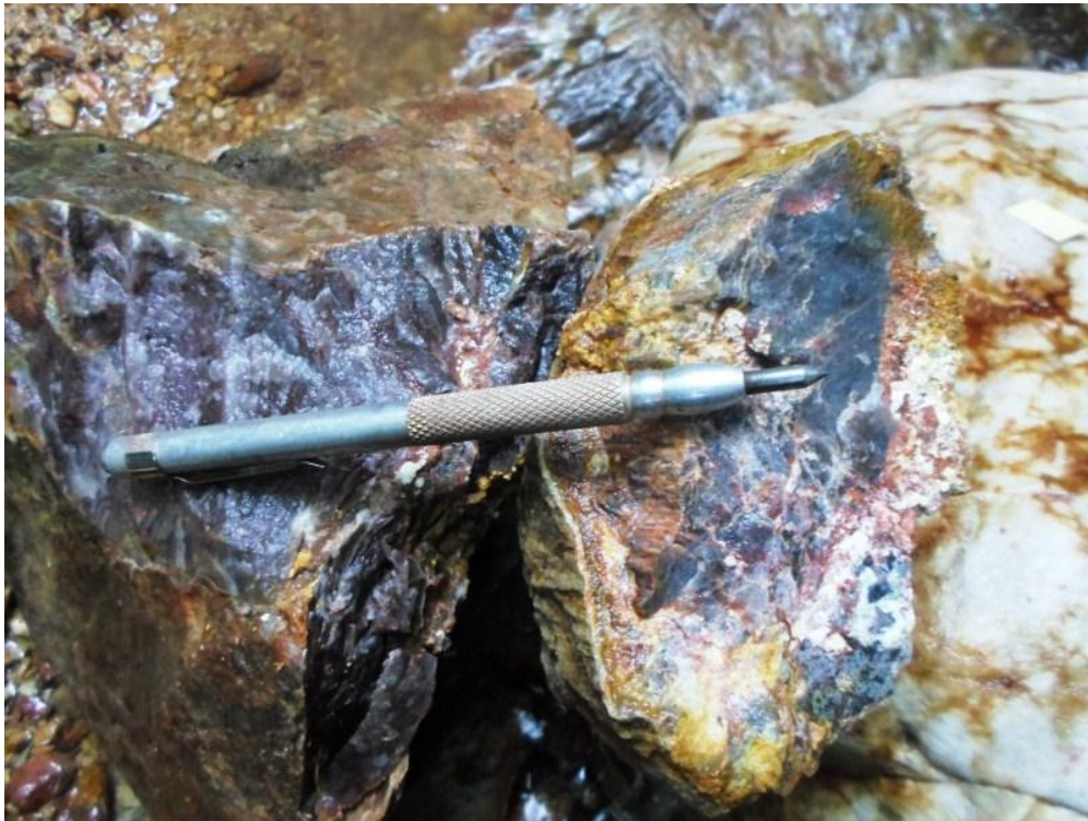
Photo 7- Sample from the Guida creek bed – banded black=stained quartz
