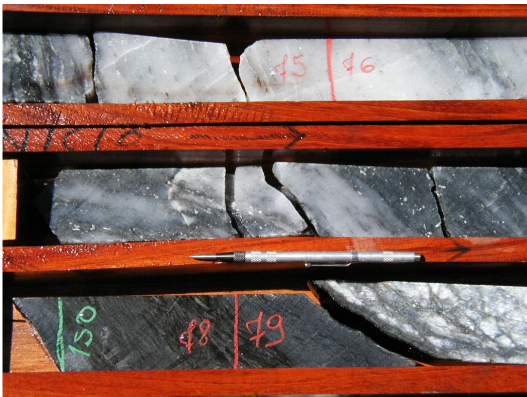
Figure 5. Typical quartz veinlets with free gold within the silicified zone of the biotite-sericite-schist
