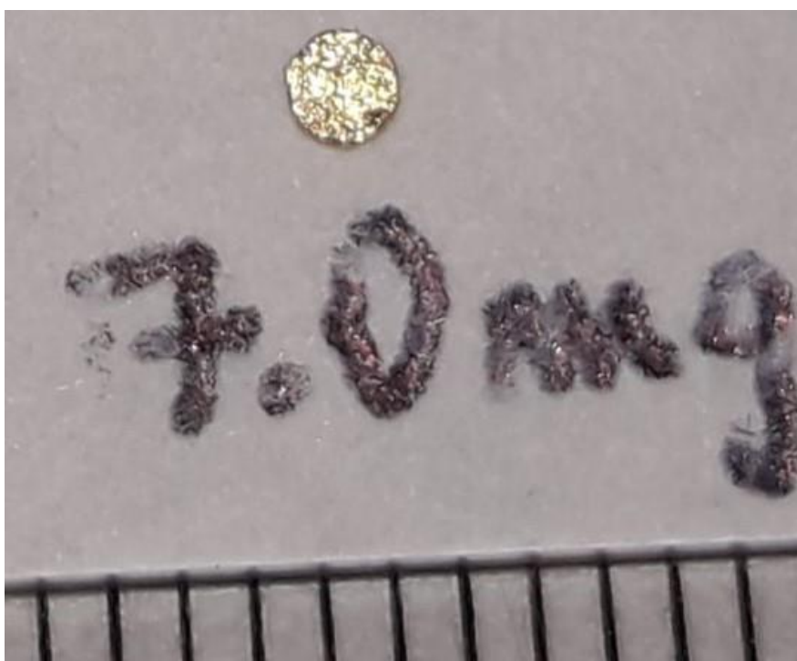
Fig. 3. Gold button recovered from 500g sample (75% of the slag utilised) (scale divisions are 1mm)
