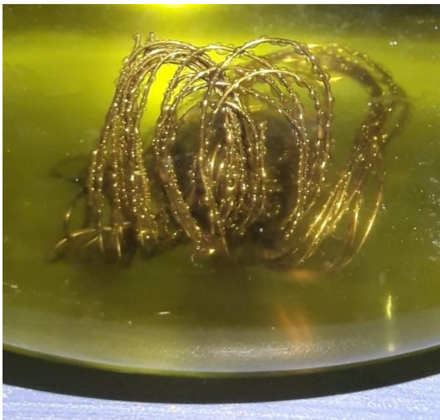
Fig. 2. Gold precipitated on copper wire from MIBK solution
