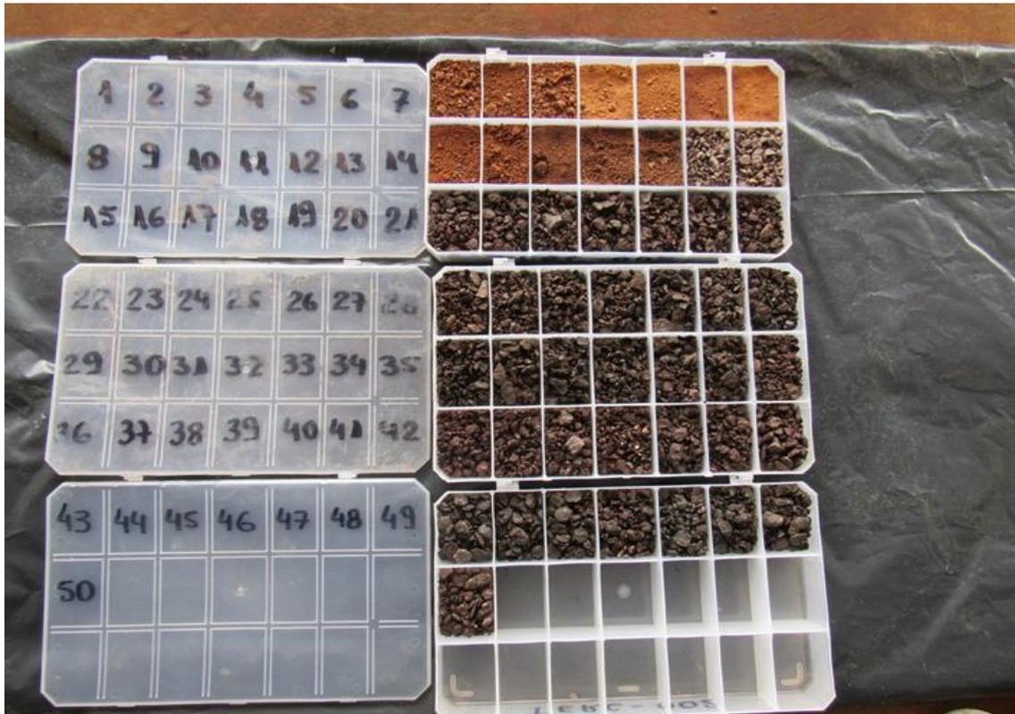
Fig. 2. One metre RC chip samples from hole TERC 02, showing fresh gabbro from 13m.
