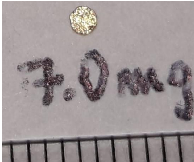
Fig. 5. Gold button recovered from 500g sample (75% of the sl utilised) (scale divisions are 1mm)
