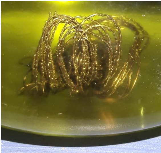
Fig. 4. Gold precipitated on copper wire from MIBK solution
