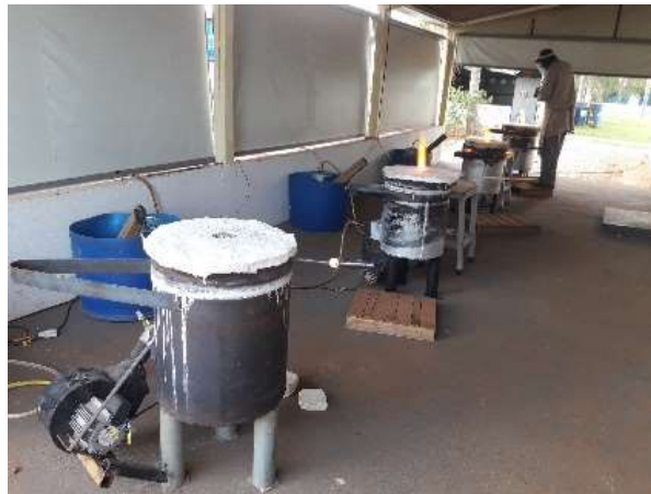
Figure 10: Furnaces in nickel smelting area
