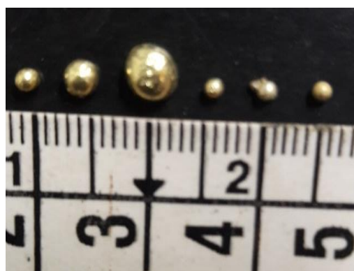
Fig. 2. Photograph of gold buttons recovered after cupellation of Ema and Tres Estados bulk samples (from left to right: EMB-3, EMB-4, EMB-5, TEB-4, TEB-5, TEB-6).
