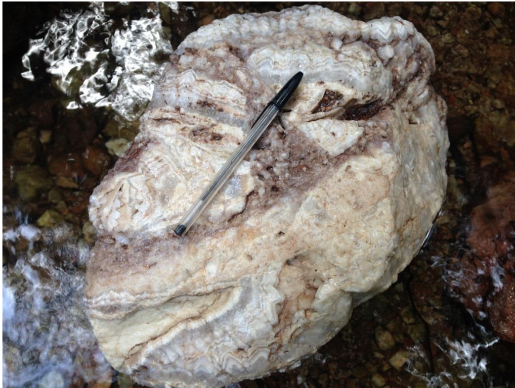
Photo 2 – 217211E/9260564N – RL 149m, Colloform sílica texture – typical of low sulphidation Au-Ag systems, between Guida and Plato targets.
