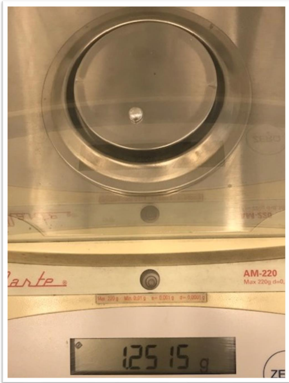
Fig. 2. Silver button recovered from copper collector
