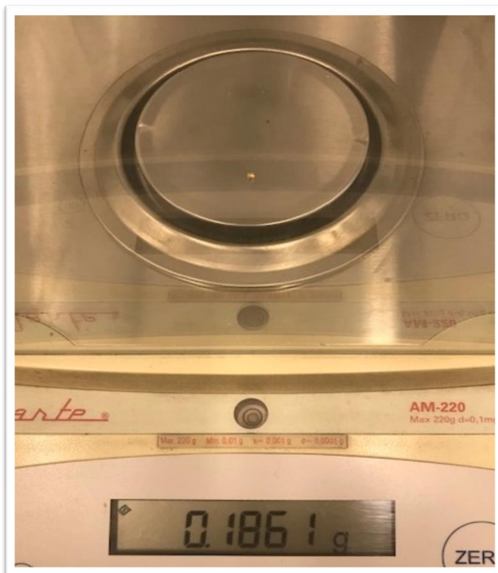
Fig. 1. Gold button recovered from copper collector
