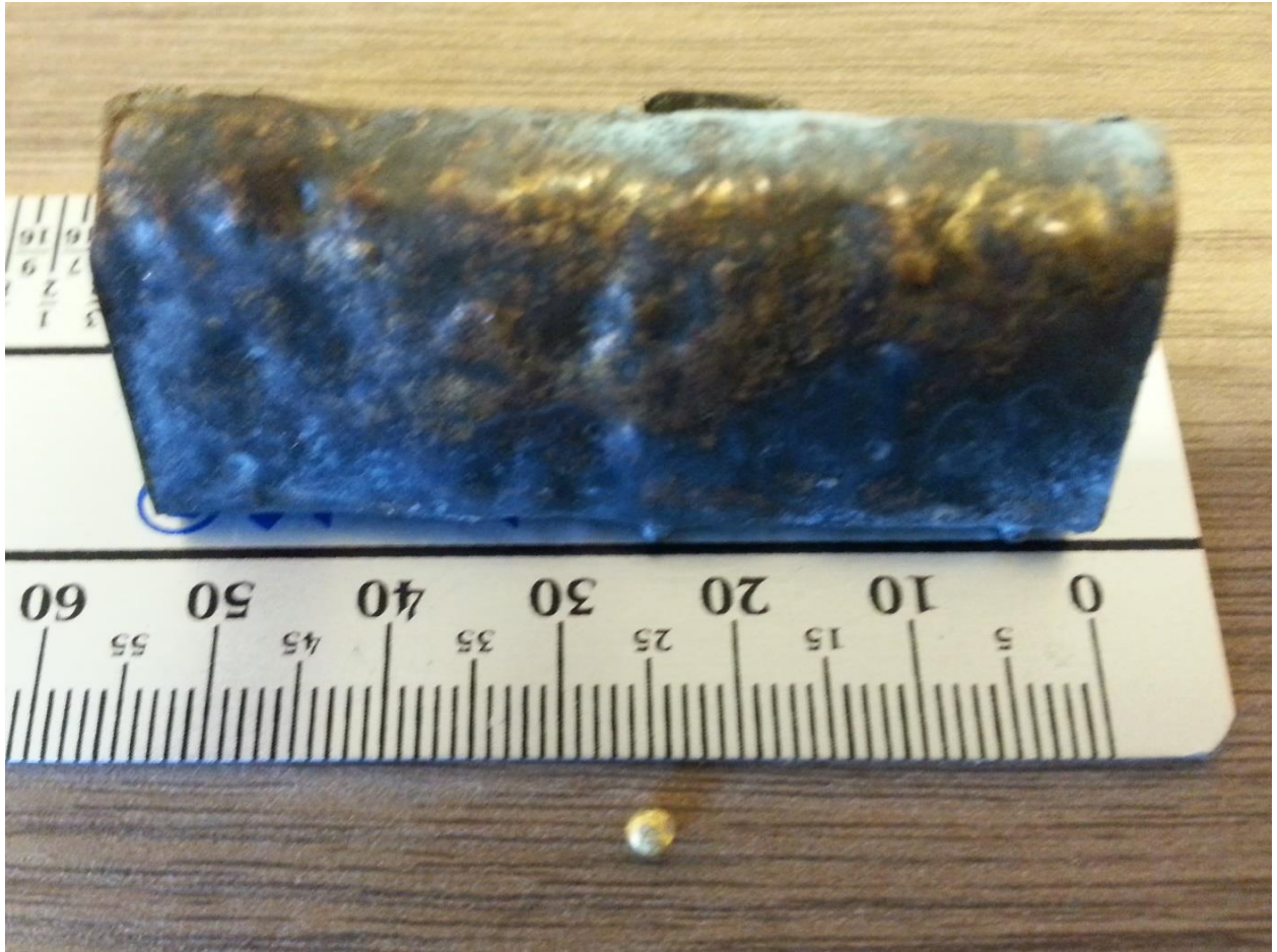
Fig1. Example of a one quarter copper bar and extracted gold button (TERC-003, 14-16m)
